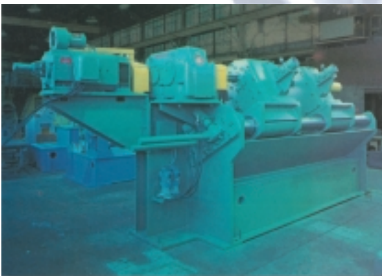
Size D11 double reduction, "limited backlash" design on a Scrap Chopper.
