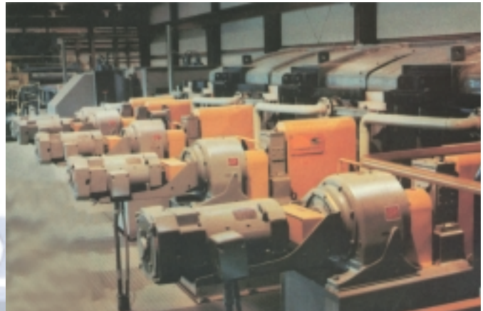
Squeegy Roll drives combining a size U54D "Moduline®" concentric gear reducer with a PS6 vertical offset parallel shaft splitter drive.
