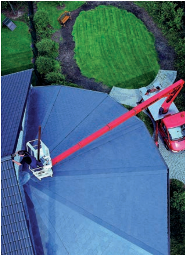
When positioning a sky lift basket, using smart actuators makes it possible to limit movements and avoid potential dangers.
